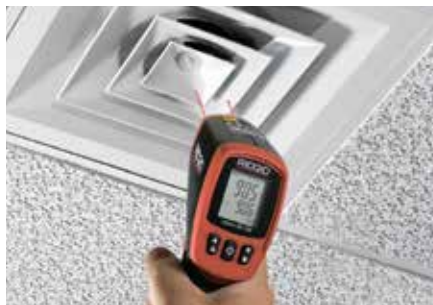
Measure efficiency of heat dissipation to reveal and locate thermal losses in flow systems
