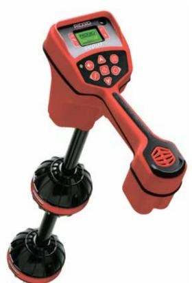
The NaviTrack Scout locator is designed to solve the most demanding remote transmitter (sonde) locates using multi-directional locating technology.
