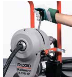
Release handle, cable stops instantly
