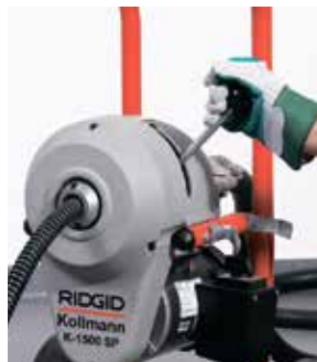
Engage clutch, cable spins
